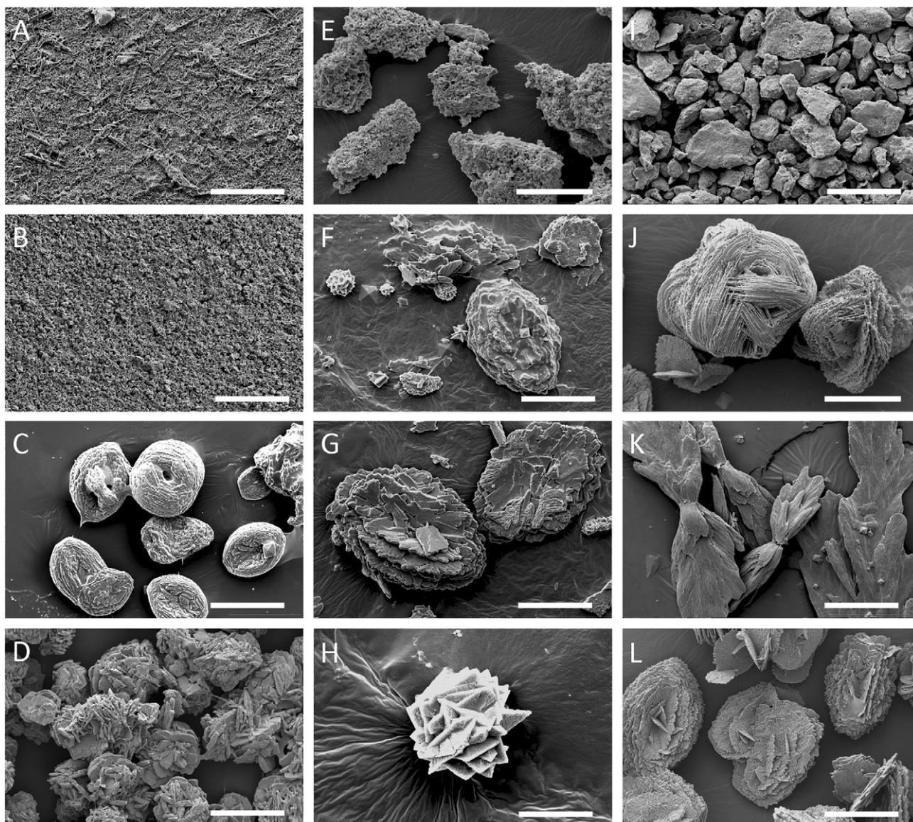
**Fig. 2.** Scanning electron microscopy of manganese oxides and the biominerals extracted from manganese oxide-amended MEA after fungal growth on (A–D)  $\text{MnO}_2$  and  $\text{Mn}_2\text{O}_3$  (E–H) biogenic  $\text{MnO}_x$ , and (I–L) birnessite.
