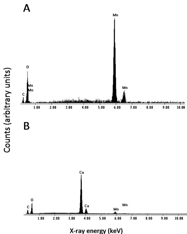
**Fig. 3.** X-ray microanalysis of crystals produced by *Aspergillus niger* and *Serpula himantioides* during growth with biogenic  $\text{MnO}_x$ . A. Manganese-containing biominer produced by *S. himantioides*. B. Calcium-containing biominer (shown in Fig. 2H) produced by *A. niger*. Typical spectra are shown from one of at least three determinations.
