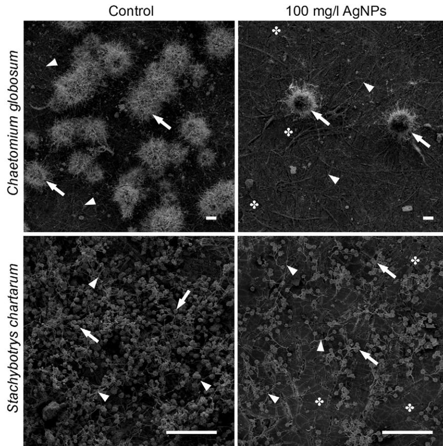
**Fig. 5.** Fruiting bodies and conidiophores (arrows) of *Chaetomium globosum* and *Stachybotrys chartarum*, respectively, present on the surface of the gypsum wallboard when fungi were treated with 100 mg/l of AgNPs (right panel) or untreated (control; left panel). Hyphae of fungi covering and penetrating the paper surface are well visible (arrowheads). ✱ indicates places when the paper surface is degraded due to the presence of fungi. Scale bar: 280  $\mu$ m.
