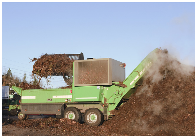
Fig. 3 – The release of A. fumigatus conidia and other bio-aerosols during the grinding of organic waste at an industrial composting facility. Credit: Ezzoom/Dreamstime.com.
