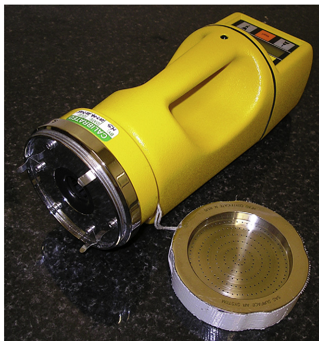
Fig. 2 – An SAS Super 180 air sampler showing the 219-hole sieve head plate, through which air is aspirated over mycological agar in a 90 mm Petri dish.
