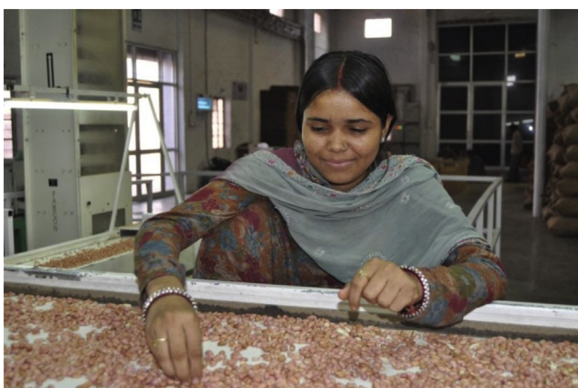
Fig. 3. Groundnut kernels passing along a conveyor belt during hand picking – Gudjurat province, India. Photograph courtesy of M. Szabo-Vezse.
