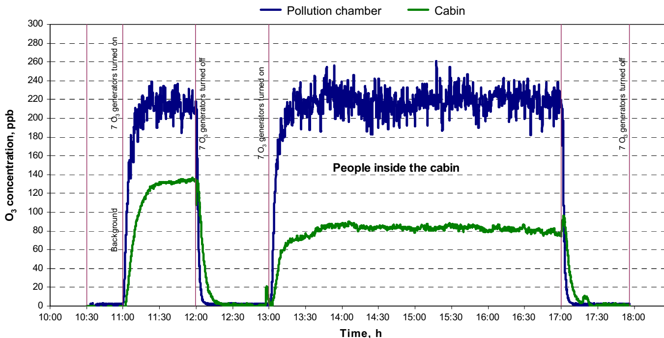
Fig. 2 Ozone levels in the pre-chamber (pollution chamber, upper trace) and simulated aircraft cabin (lower trace) on the day of an ozone experiment. During this example, the air exchange rate was 8.8 \text{ h}^{-1}
