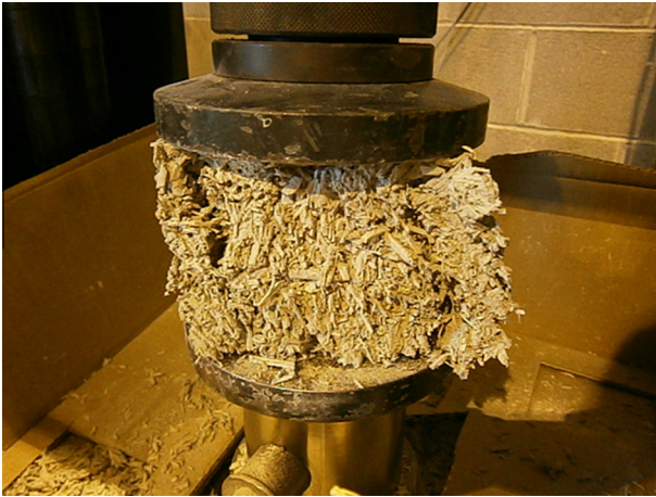
Fig. 5. Typical failure of hemp-lime concrete under an axial compressive load.
