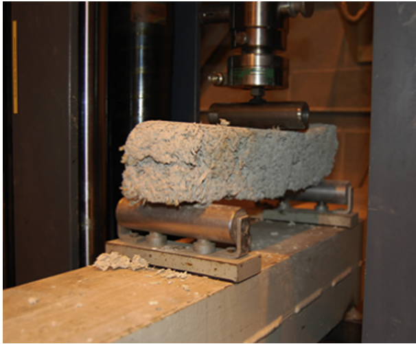
Fig. 8. Typical deflection of hemp-lime concrete in bending.
